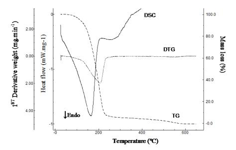
**Figure 2**. DSC and TG/DTG curves of OEHP in dynamic nitrogen atmosphere (50 mL.min<sup>-1</sup>) and heating rate 10°C.min<sup>-1</sup>from *H. fruticosa* essential oil.
